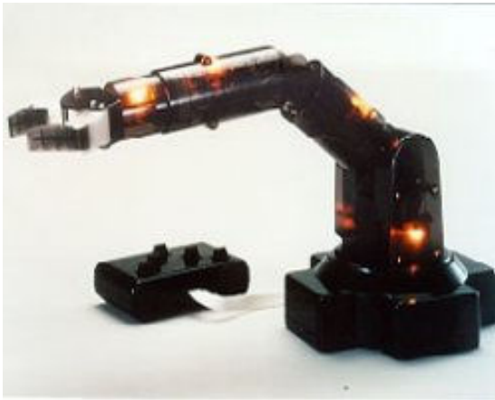
Fig.2 The previous image illustrate the final assembly of the Articulated Robotic Arm (OWI-007) and Remote Control Box
